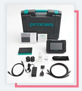
Ultrasonic Pulse Velocity Tester (Pundit Lab +)
