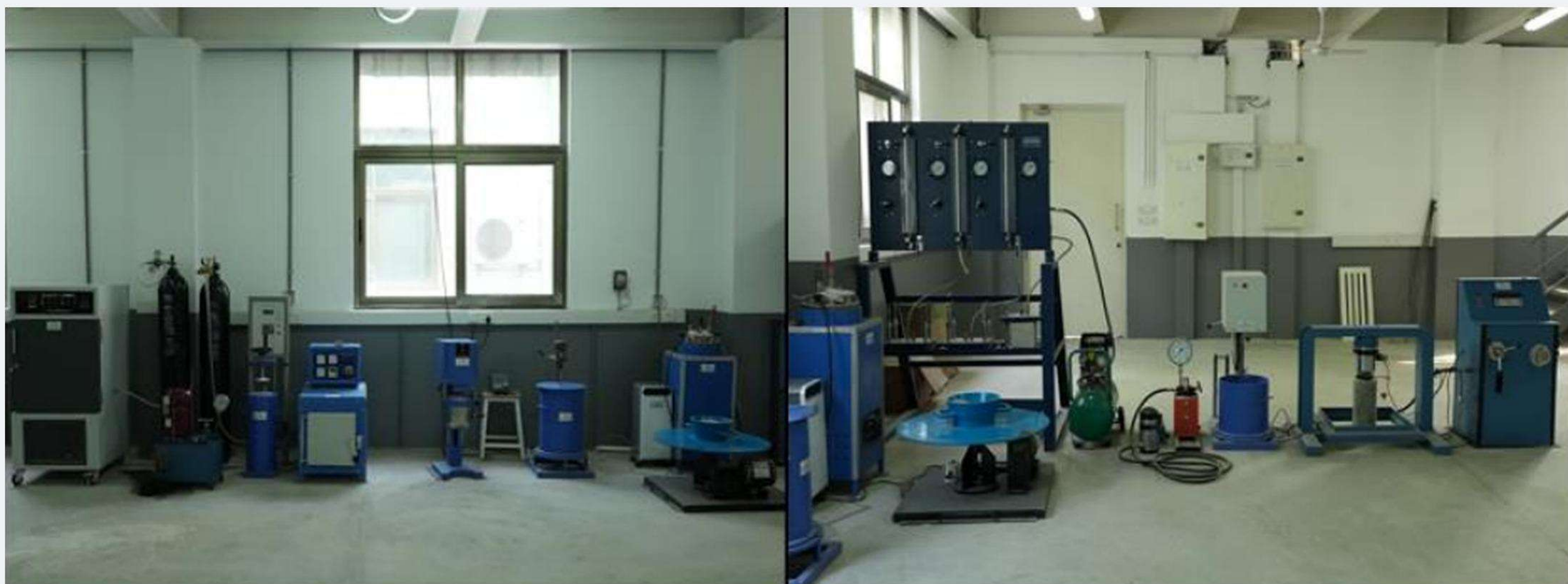
Fig. 3. New Lab Equipment - Humidity Chamber, Mortar Mixer, Vibration Table, Permeability, Shotcrete Impact, Muffle Furnace, Mist Generating Unit. (From Left to Right)
