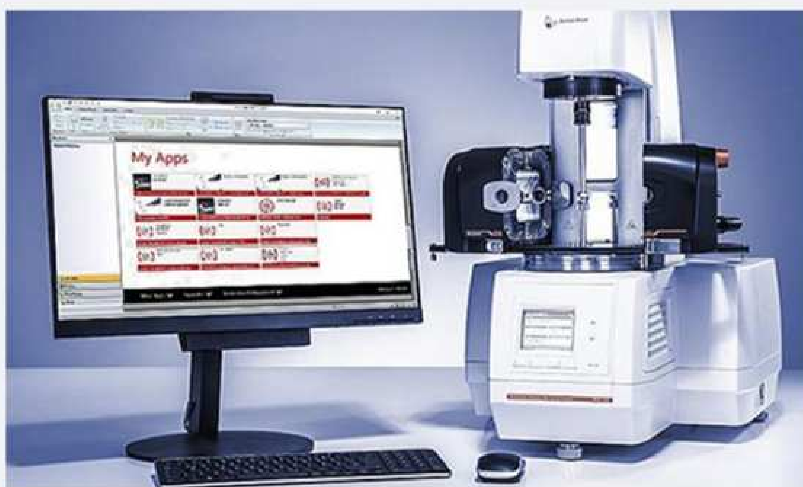
Fig. 2. New Lab Equipment - Dynamic Shear Rotometer, Combined Environmental and Mechanical Loading Chamber
