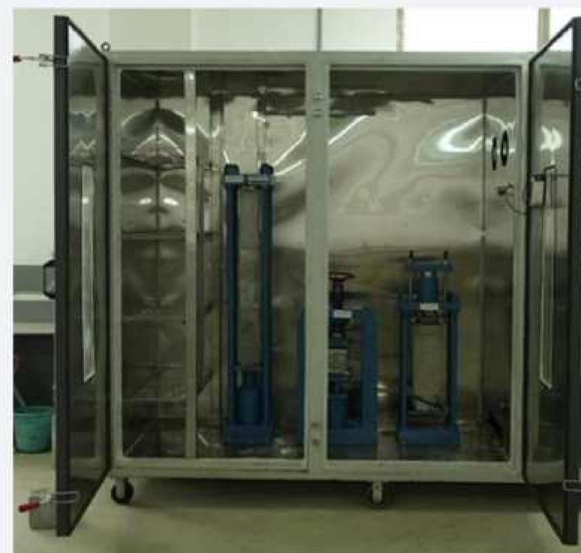
Fig. 2. New Lab Equipment - Dynamic Shear Rotometer, Combined Environmental and Mechanical Loading Chamber
