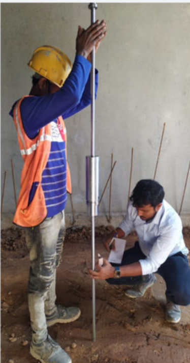
Fig. 3. Pictorial view of DCPT on the compacted surface.
