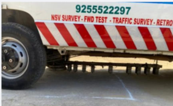
Fig. 7. Pictorial view of FWD-NDT device on controlled section in the field.
